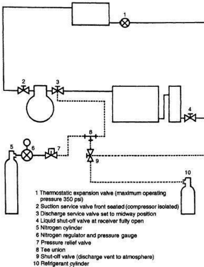
*Typical test arrangement for leak testing at 300 psi*
