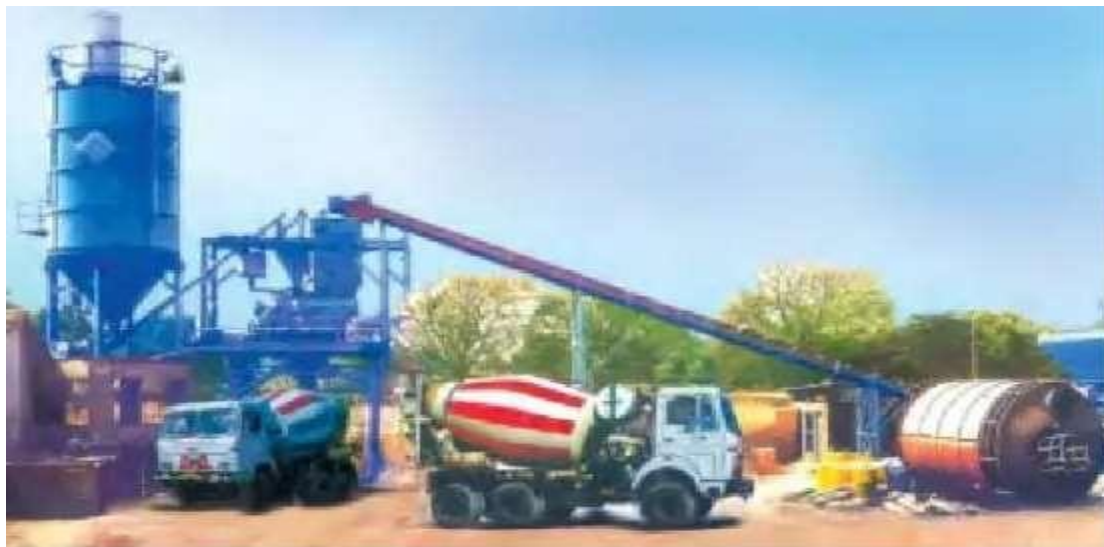
Modern ready mixed concrete plant.
