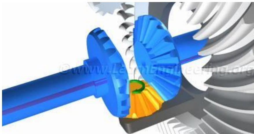
Fig.8 While taking left turn the spider gear spins in opposite direction
