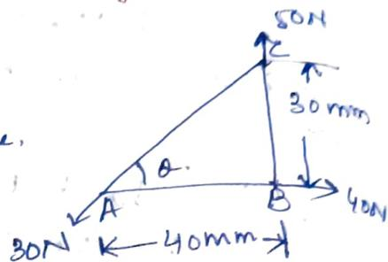
Q. A system of forces are acting at the corners of a rectangular block as shown in fig 2.4.
