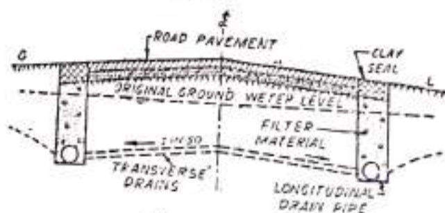
SUB-SURFACE DRAINAGE WITH TRANSVERSE DRAINS ALONG WITH LONGITUDINAL SIDE DRAINS
