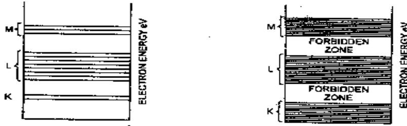
Figure -3.3 (b) Energy band representation of ionisation
