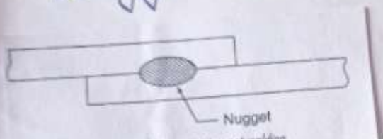
Fig. 9.61 Formation of a nugget in spot welding
