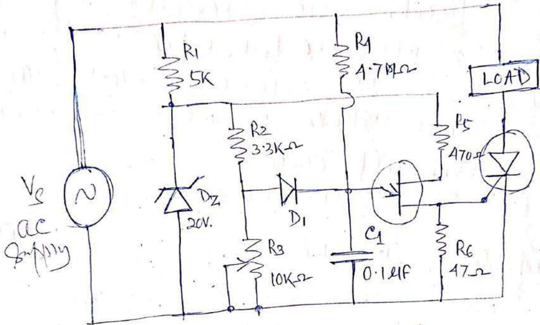
As the fig. is shown the UJT-SCR control circuit in which the ramp-pedestal structure of emitter voltage is utilized to produce triggering pulses.
