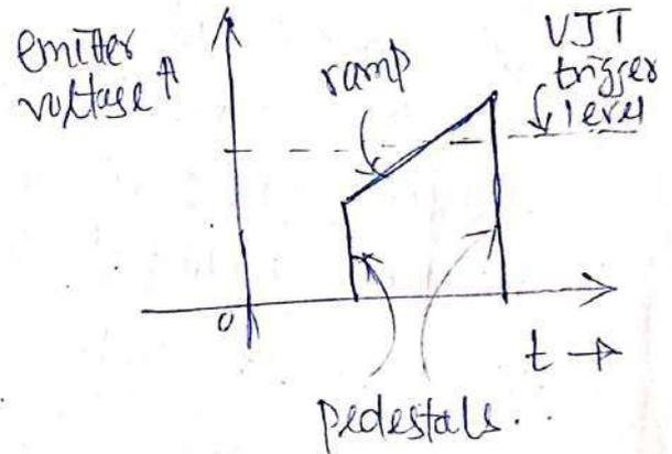
When the supply voltage exceeds 20V, the Zener diode conducts, providing a dc voltage across the base connection of UJT. At the same time diode  $D_1$  is forward biased and capacitor  $C_1$  charges quickly through  $R_1$  &  $R_3$ . This represents the left hand pedestal portion of the emitter voltage once the capacitor charges to the voltage across  $R_3$ ,  $D_1$  will become reverse biased.
