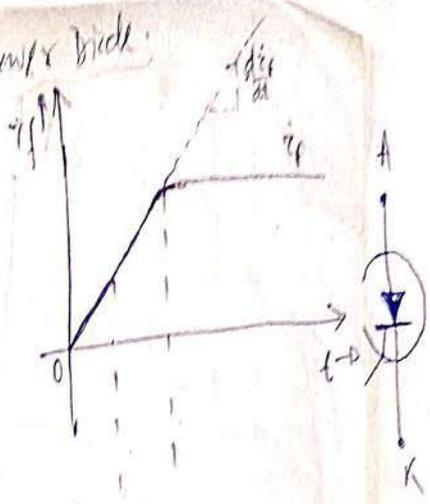
Forward current increases from its initial value (0) and reaches a steady state value of  $i_f$ .
