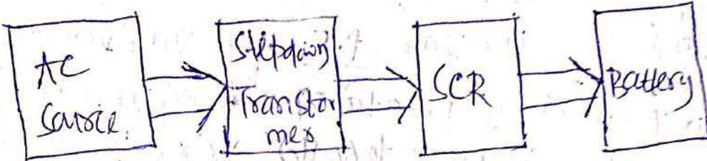
AC supply is given to a stepdown transformer which converts large ac voltage to lower ac voltage. Then it is filtered to remove noise and then rectified by an SCR. The rectified dc voltage is used for charging the battery.
