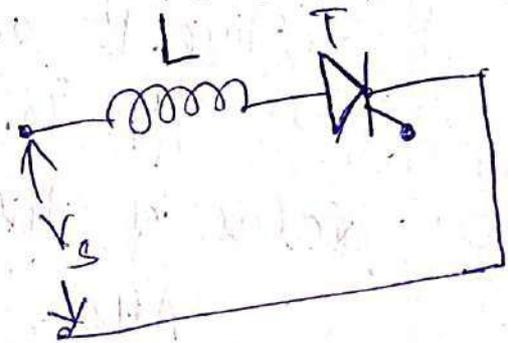
with the SCR. When current variation is high, the inductor opposes it or smooths it and protects the SCR.
