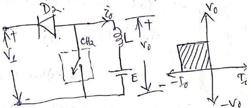
when  $CH_2$  is ON:  $v_o = 0$ , but the load voltage  $E$  drives the load current through inductor  $L$  and  $CH_2$  in the direction opposite to that shown in figure, so  $i_o$  is -ve. During this ON period the inductor gets charged.
