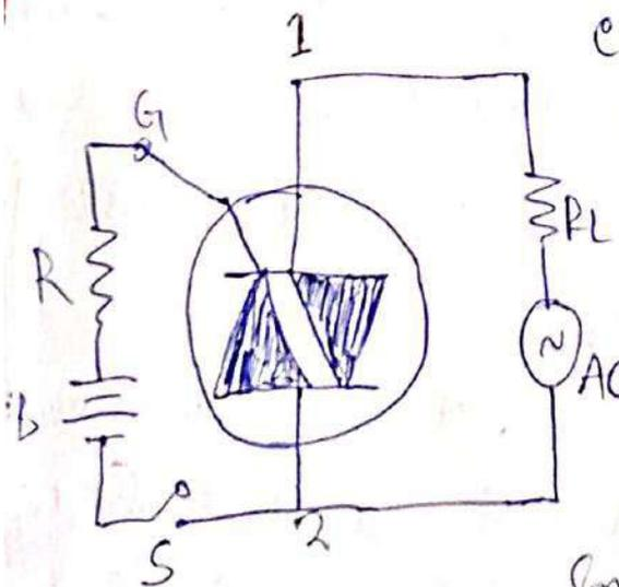
in the fig. is shown the simple triac ckt. The ac signal to be controlled is applied between the two anodes through a load resistor PL. The gate ckt consists of a battery B, a current limiting resistor R and a switch S. without gate supply, the triac can be triggered
