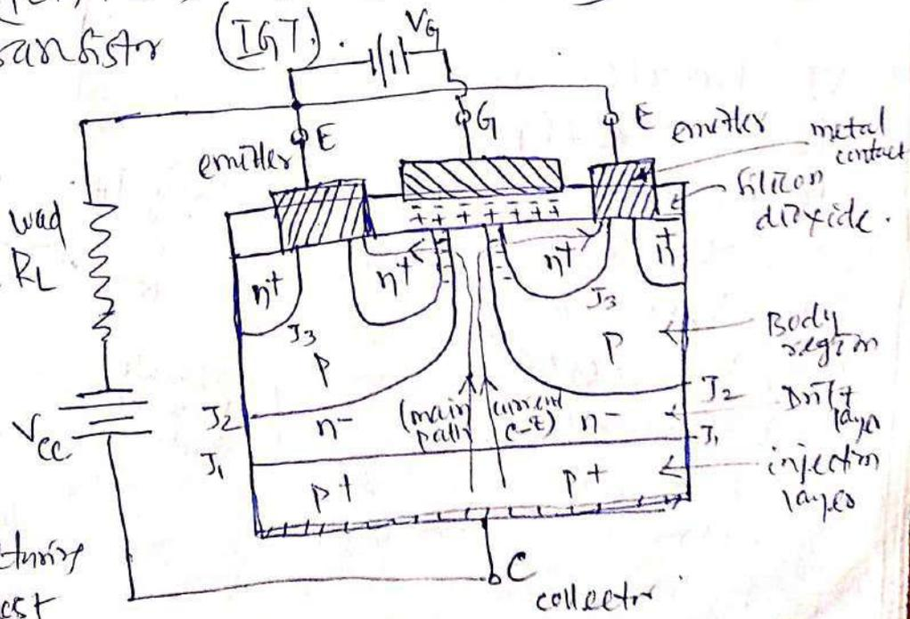
on the fig. of given the basic structure of an IGBT. The manufacturing process is almost
