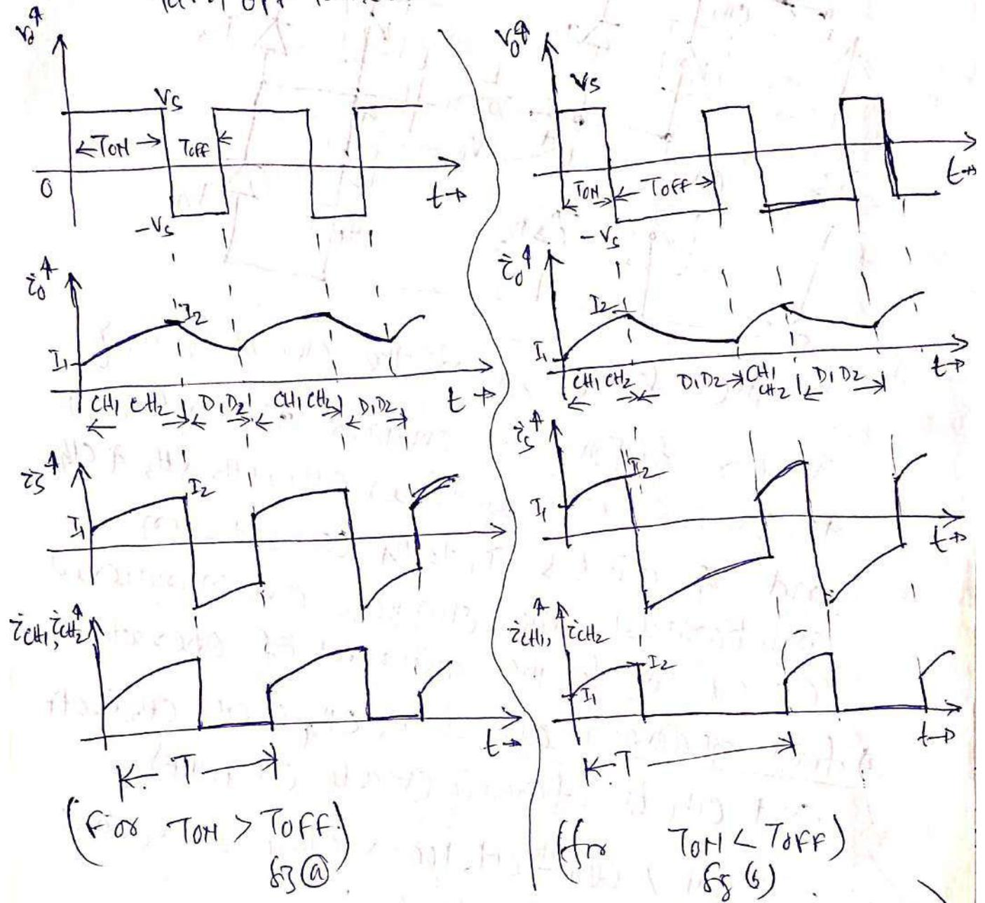
for  $T_{on} > T_{off}$ , the various waveforms are plotted in fig (a); average values of both  $v_o, i_o$  (that is  $v_o, i_o$ ) are both +ve and chopper operates in 1st quadrant power flow takes place from source to load.
