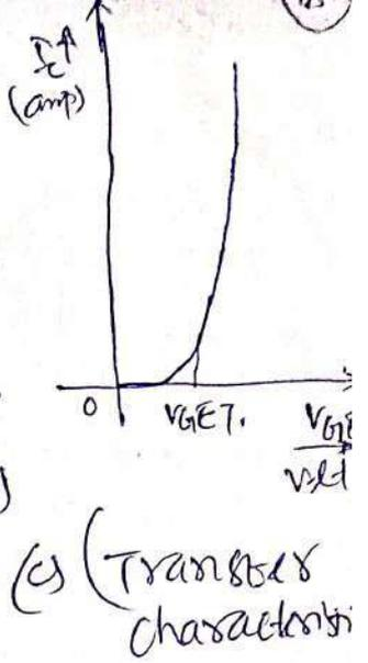
gate to emitter voltage constant. In forward direction, the characteristics resemble to that of a BJT, but the controlling parameter is the gate-to-emitter voltage  $V_{GE}$ . In reverse direction  $V_{RM}$  is the maximum reverse breakdown voltage.
