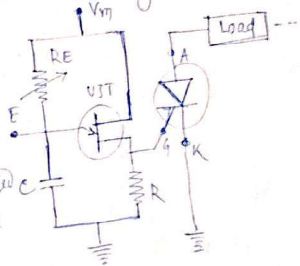
The resistance  $R_E$  is so chosen that the load line determined by this resistance  $R_E$  passes through the device characteristic curve in the -ve resistance region, between peak point ( $P_p$ ) and valley point ( $P_v$ ).
