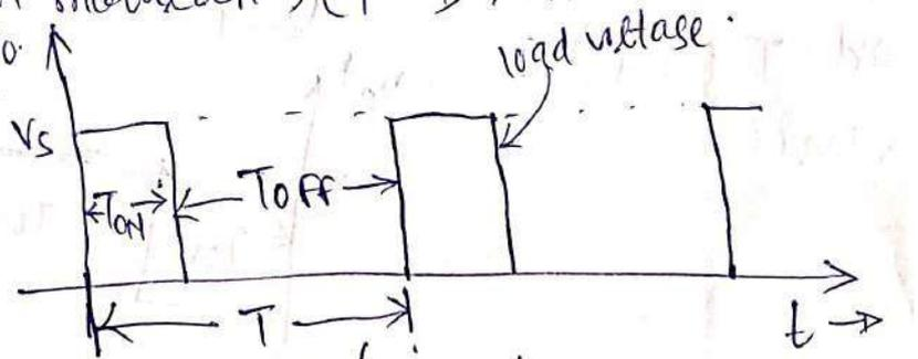
Fig (a) ( $T_{on} = \frac{1}{4}T$  or  $d = 0.25$  or 25%)
