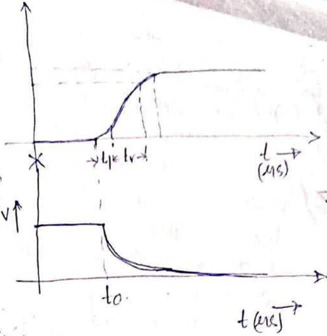
$t_0$  indicates the initiation of turn ON, which is caused by applying a step voltage to the gate.
