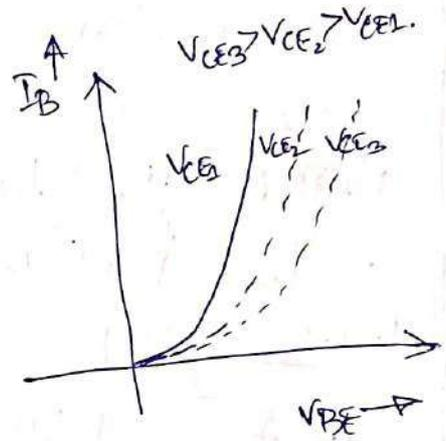
As the input ckt is simply a forward biased PN junction (base to emitter), the input characteristic is the forward biased diode characteristic. Now changing  $V_{CE}$  to different values, a number of ch. curves can be drawn.
