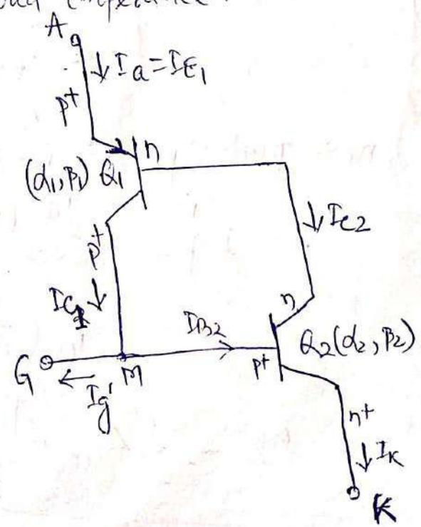
for transistor  $Q_1$ ,  $I_{C1} = d_1 I_E1 = \beta_1 I_{B1}$
