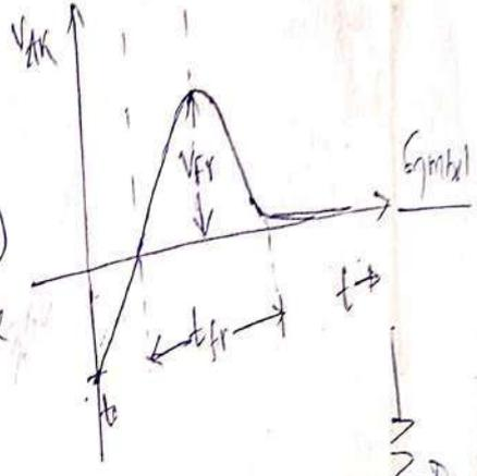
Forward diode voltage  $V_{AK}$  (anode to cathode voltage) rises from a -ve value to a maximum value  $V_{FR}$  called forward recovery voltage and is given as a function of rate of change of forward current i.e.,  $\frac{di_f}{dt}$ .
