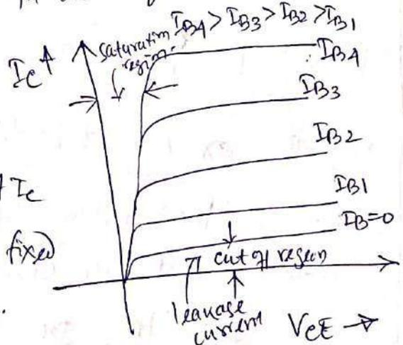
For small values of  $I_B$  (for  $I_B = 0$ ), the collector current is very small ( $\approx 0$ ). This is small value of
