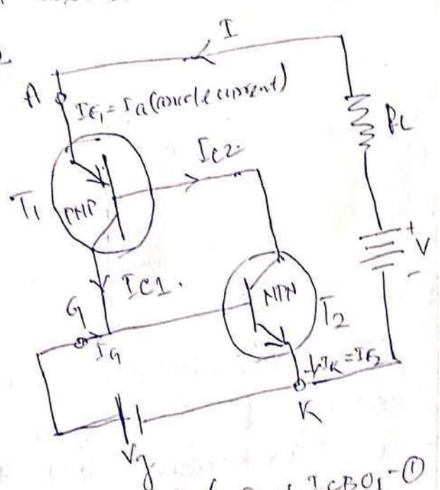
for the transistor  $T_1$ ,  $I_{c1} = \alpha_1 I_a + I_{cBO1}$  — ①
