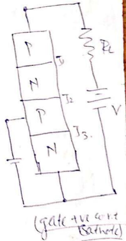
The operation of SCR can be explained with the conditions a) gate open b) gate is +ve w.r.t. cathode when gate is open — as anode is at higher potential than cathode junctions  $J_1$  &  $J_3$  are F.B. and  $J_2$  is reverse biased. So the SCR is OFF or non-conducting. But increasing the anode
