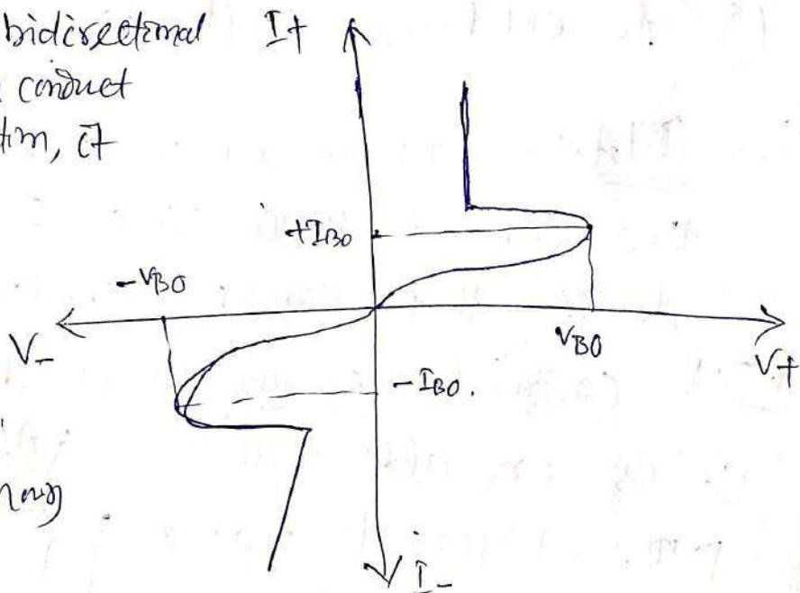
When a voltage (+ve or -ve) is applied less than the breakover voltage  $V_{BO}$ , a leakage current  $I_{BO}$  flows through the device. This leakage current is due to drift of holes & electrons in the depletion region. This current is not sufficient to cause conduction and device
