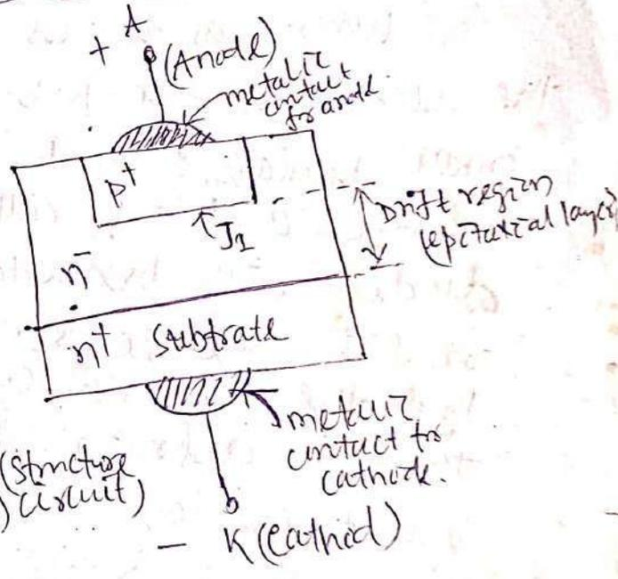
A heavily doped n+ substrate (act as cathode) over which a lightly doped n- layer is epitaxially grown. This layer is so lightly doped that it behaves as intrinsic layer and so called i-layer. To this layer
