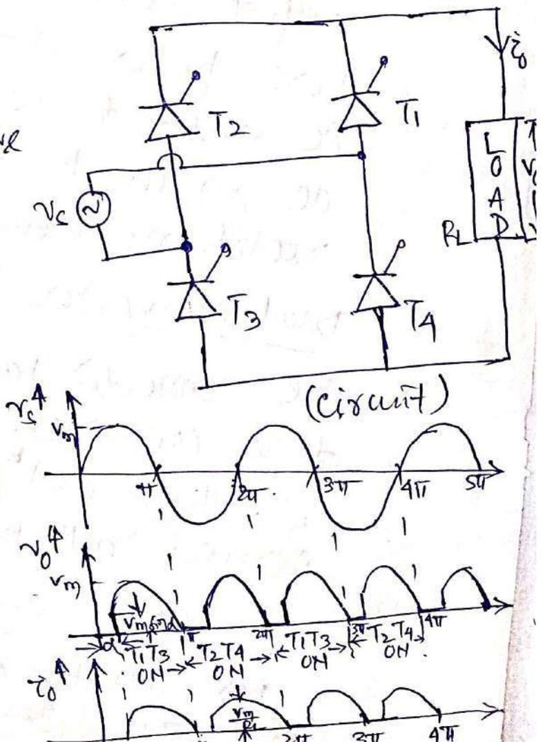
$T_1$  &  $T_3$  are fixed (conducting) and thyristors  $T_2$  &  $T_4$  are in reverse blocking state and so OFF. The thyristors  $T_1$  &  $T_3$  are fixed at angle (say  $\alpha$ ) after the reverse time ( $t=0$ ) when their anode voltage increases from '0' to +ve values.
