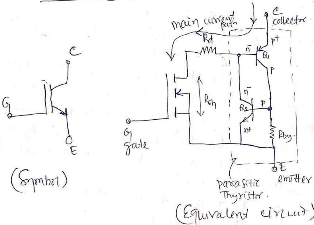
The equivalent circuit is as shown in figure. It consists of an MOSFET along with a parasitic thyristor consisting two transistors Q<sub>1</sub> & Q<sub>2</sub>. Q<sub>1</sub> is the pnp transistor and Q<sub>2</sub> is the npn transistor. R<sub>ch</sub> is the n-channel resistance. R<sub>d</sub> is the resistance offered by the n<sup>-</sup> drift region. R<sub>by</sub> is the p-type body resistance. The main current path is as shown. The next fig. shows the circuit symbol of IGBT.
