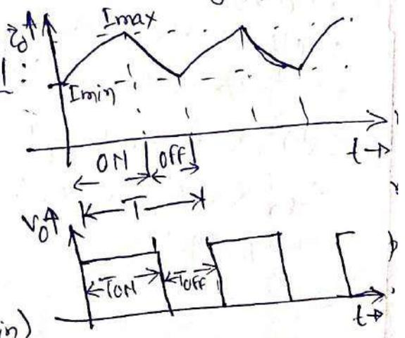
Switching freq. of the chopper can be controlled by setting  $I_{max}$  and  $I_{min}$ . The ripple is given by  $(I_{max} - I_{min})$  which can be lowered by increasing the switching frequency.
