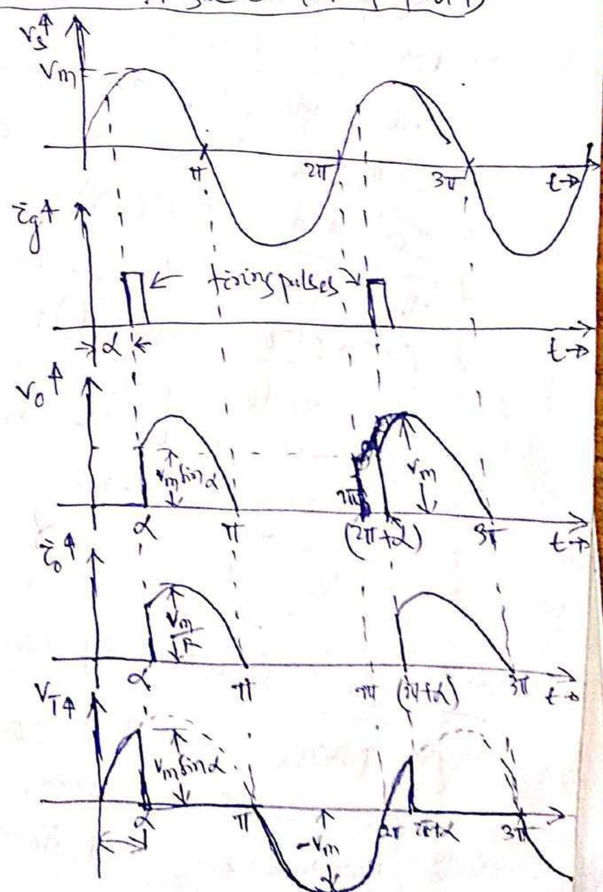
on the fig. is shown the simplest ckt. of a controlled rectifier which consists of a single thyristor providing dc power to a resistive load.
