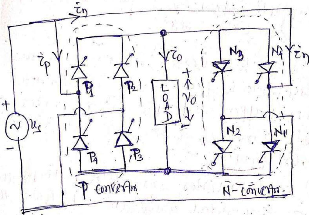
The circuit of a  $\phi$  1- $\phi$  to 1- $\phi$  cycloconverter is as shown in the figure. It consists of two full wave fully controlled bridge converter circuits using four thyristors for each bridge.
