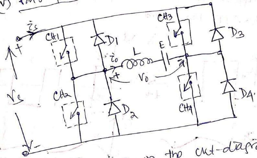
on the fig is shown the cut-diagram of a four quadrant chopper. It consists of 4 semiconductor switches  $CH_1, CH_2, CH_3$  &  $CH_4$  and 4 diodes  $D_1$  to  $D_4$  connected in anti parallel. The choppers are numbered according to the quadrant of operation.
