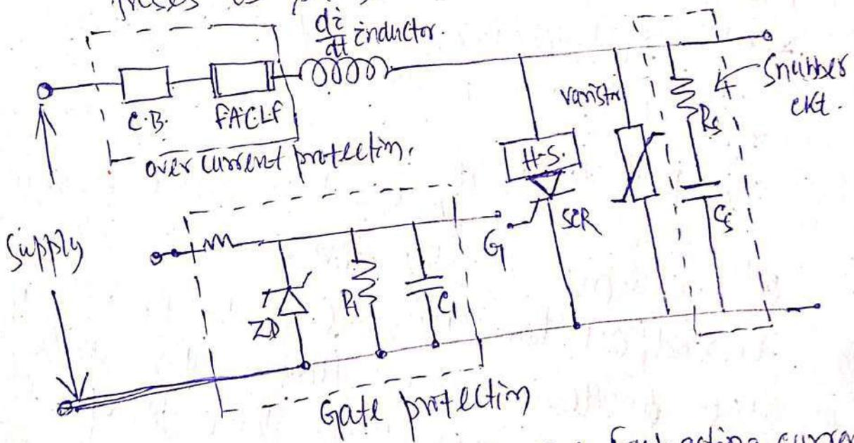
C.B.  $\rightarrow$  circuit breaker, F.A.C.L.F.  $\rightarrow$  Fast acting current limiting ~~switch~~ fuse, H.S.  $\rightarrow$  Heat sink, ZD  $\rightarrow$  Zener diode
