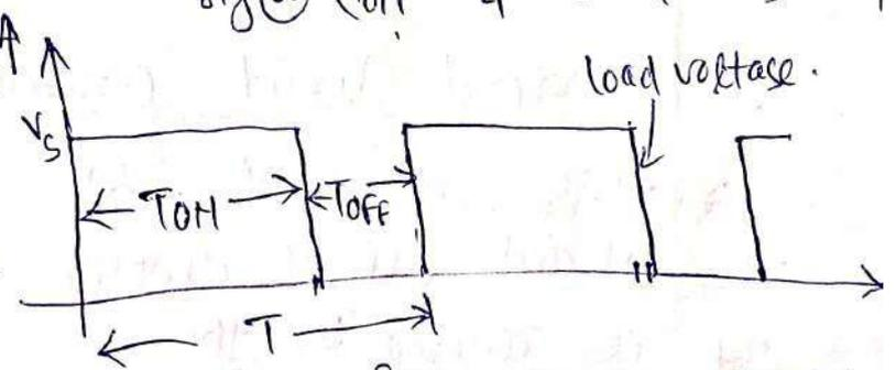
Fig (b) ( $T_{on} = \frac{3}{4}T$ , or  $d = 0.75$  or 75%)
