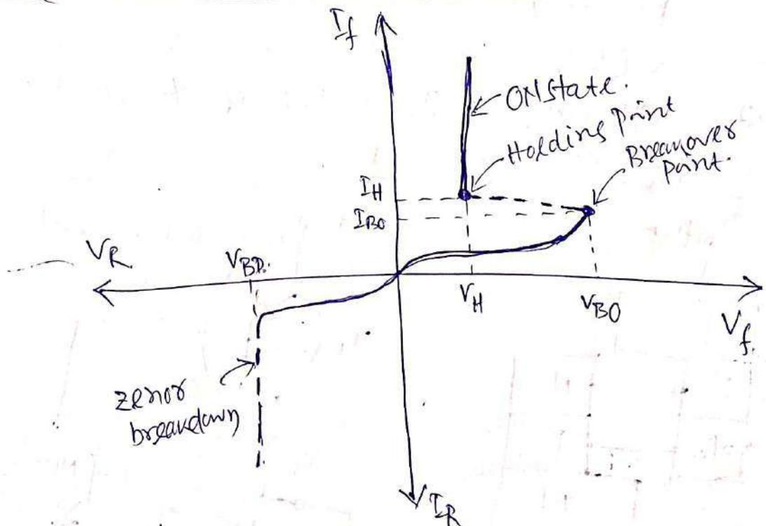
The VI characteristics of an SCR is as shown in fig for  $I_g \geq 0$ , (gate open). When anode is made +ve w.r.t cathode and the applied anode voltage increases slowly, the characteristics is called forward characteristics.
