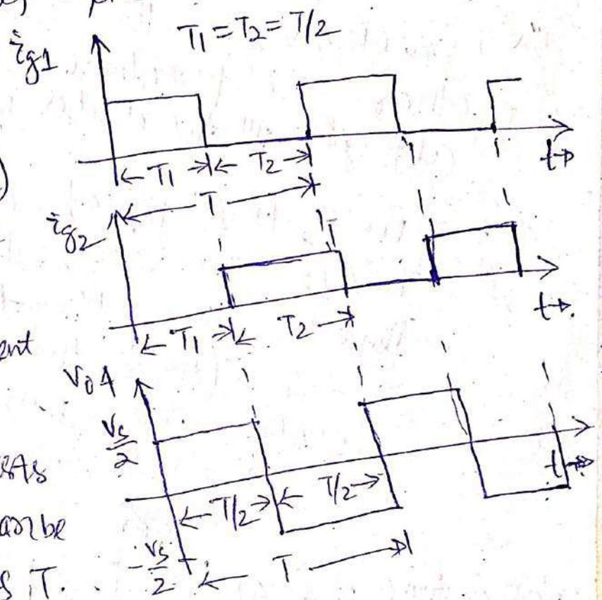
Q2 Single phase ~~full bridge~~ full bridge voltage source inverter (1 $\phi$ FBVSI)
