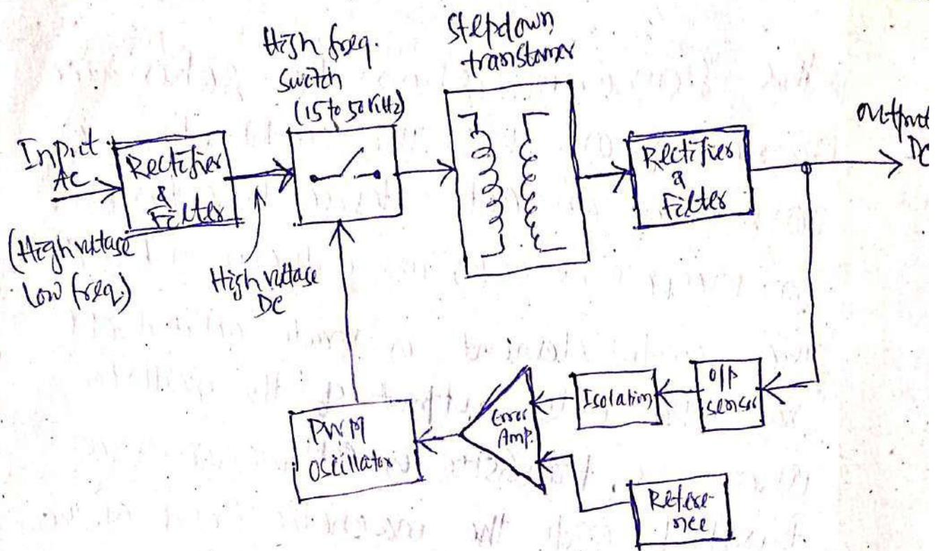
The high frequency pulse switch is driven by the PWM oscillator, its output being fed to the primary of the step down transformer. The duty cycle is made 50% that is  $T_{ON} = T_{OFF}$  (duty cycle  $\delta = \frac{T_{ON}}{T} = \frac{T_{ON}}{T_{ON} + T_{OFF}}$ ), so that maximum energy will pass through the step down transformer.
