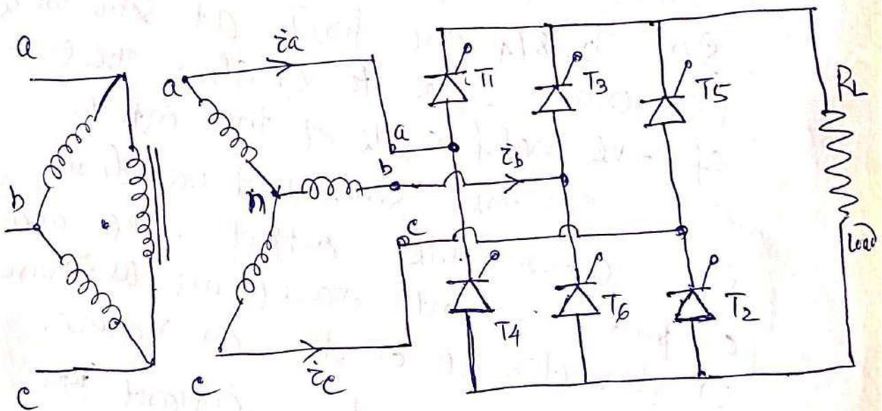
3- $\phi$  full wave controlled bridge rectifier with resistive load)
