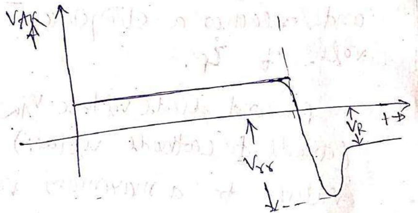
rather decreases to a -ve peak value of  $I_{RS}$  (peak reverse recovery current) and after some times (transients), it again increases to zero value. During reverse recovery the voltage across the diode decreases to the lowest possible value called  $V_{RS}$  (reverse recovery voltage and again increases to remain steady at  $V_R$  (reverse bias voltage).
