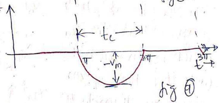
As the supply voltage is ac, it has its natural -ve going half cycle (zero crossing) which when applied to the thyristor, it
