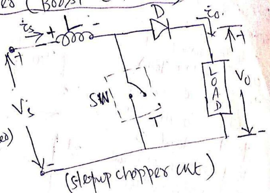
( $0 \leq t \leq T_{on}$ ), the inductor get charged by  $V_s$  and load cut is cut off from the supply. So the output  $V_o = 0$ .
