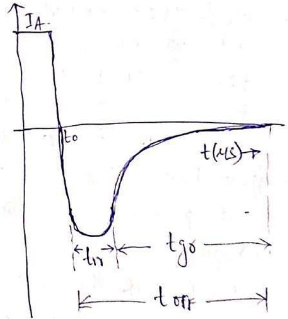
$t_0$  indicates the instant of application of reverse voltage.  $t_{rr}$  (reverse recovery time) is the duration for which recovery current flows after the application
