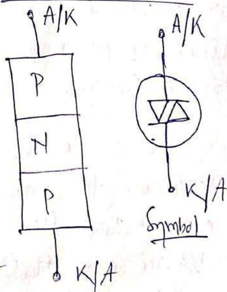
The switching from off to on state can be achieved by simply exceeding the avalanche breakdown voltage in either direction. From structural features and logic symbol it is seen that, it can be considered as an inverse parallel connection of two SCRs without control gate.
