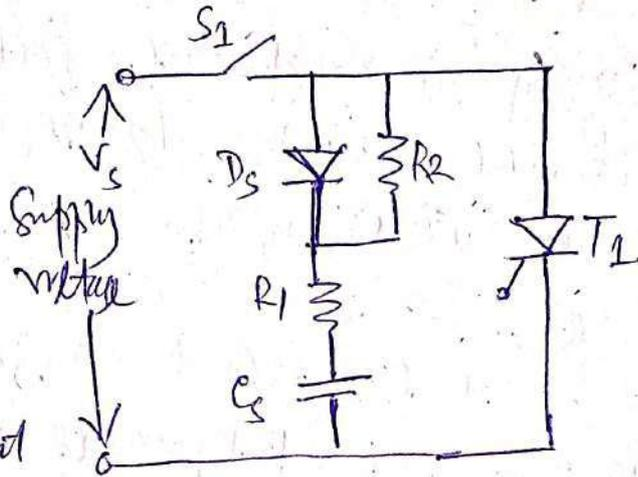
~~over~~  $\frac{dV}{dt}$  protection and  $(R_1 + R_2)$  for limiting the capacitor discharge current.
