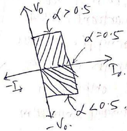
So the fig. is showing the two quadrant class B chopper or class D chopper.
