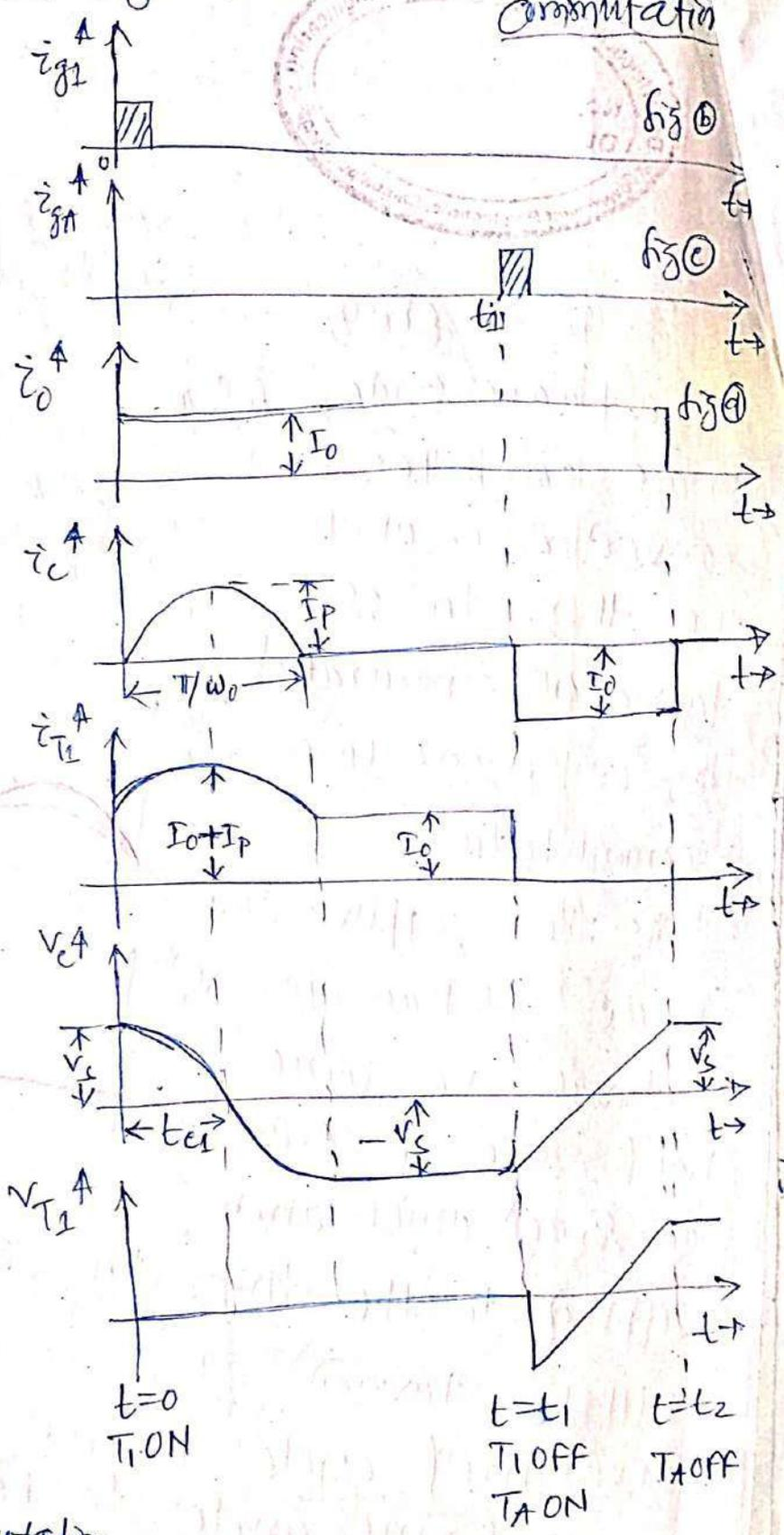
from the fig. it shows a main thyristor  $T_1$ , which is turned off with the help of an auxiliary thyristor  $T_A$ , by applying a sudden -ve voltage at its anode. Therefore it is called Auxiliary commutation or voltage commutation.
