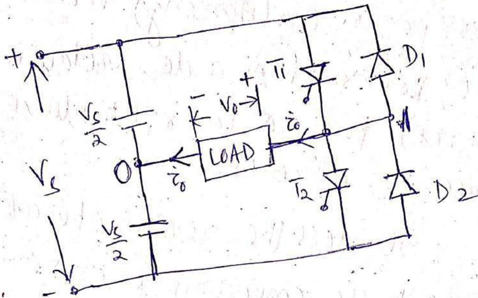
From the fig. is shown the basic circuit diagram of a 1 $\phi$  half bridge voltage source inverter. At the first stage the source voltage  $V_s$  is divided into two equal halves of  $\frac{V_s}{2}$  each through a potential divider network (maybe capacitive). To each half voltage path are connected one power switch (thyristor or IGBT or GTO) in anti-parallel with a diode. Between the junction of the bridge (point A) and junction of the two voltage halves (point O) is connected the load.
