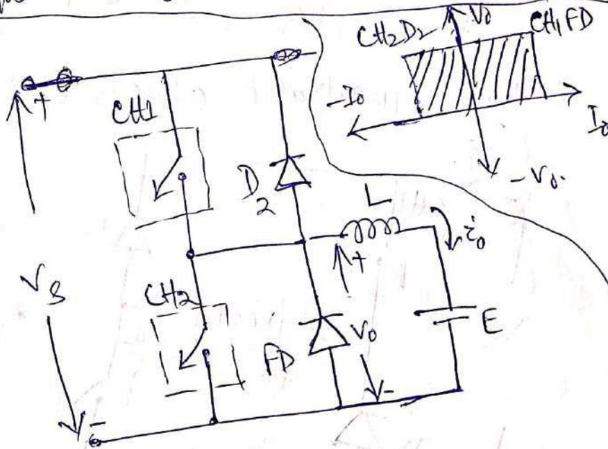
The output voltage  $v_o$  is always +ve because of the presence of the freewheeling diode FD across the load.
